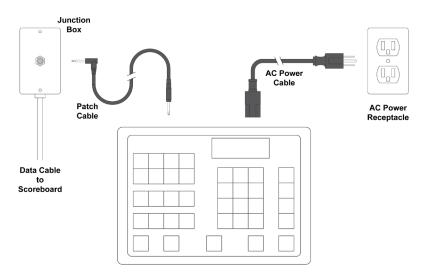
If your scoreboard package includes a ScoreLink RF Communications system, the power receptacle may be the only consideration on the control console side of the installation process. For details about ScoreLink, consult the documentation that ships with the product. Otherwise, use the stereo patch cable to plug the console into the junction box.
